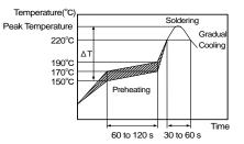
[Allowable Reflow Soldering Temperature and Time]
