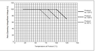
Derated products\*1 are suitable for use in circuits where continuous applied voltage and temperature to the
