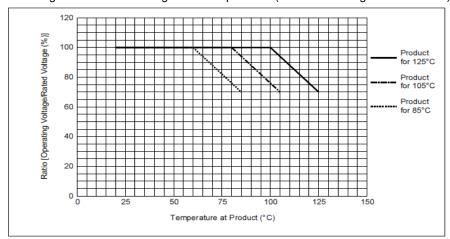
Derated products\*1 are suitable for use in circuits where continuous applied voltage and temperature to the capacitor is derated (below rated voltage and temperature).
