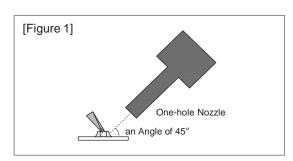
3. Optimum solder amount when re-working with a soldering iron
