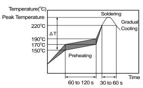
[Allowable Reflow Soldering Temperature and Time]
