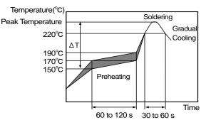
[Allowable Reflow Soldering Temperature and Time]
