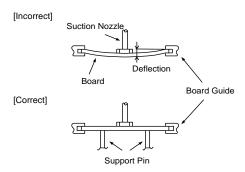
2. Dirt particles and dust accumulated in the suction nozzle and suction mechanism prevent the nozzle from moving smoothly. This creates excessive force on the capacitor during mounting, causing cracked chips.
