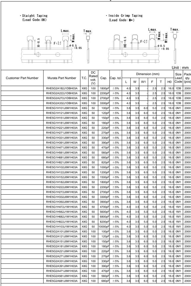
Inside Crimp Taping (Lead Code: M\*)
