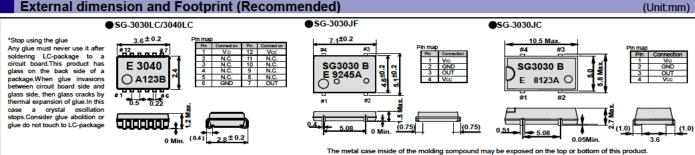
The metal case inside of the molding compound may be exposed on the top This purely cosmetic and does not have any effect on quality, reliability or el
