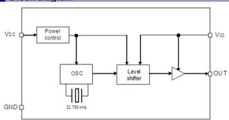
Vio is a power supply pin for OUT output and can also be used as an OE pin. Set Vio to 0 V when setting Disable.
