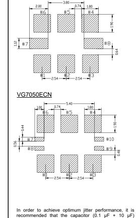
between VCC and GND pin should be placed as close to
