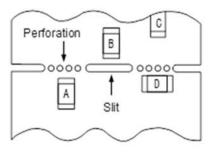
(3) Mounting components near screw holes
