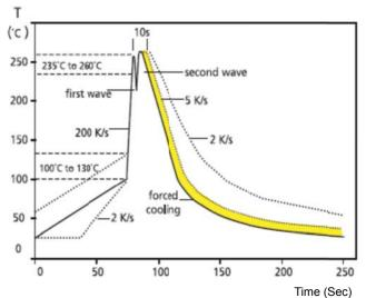
Recommended IR Reflow Soldering Profile
