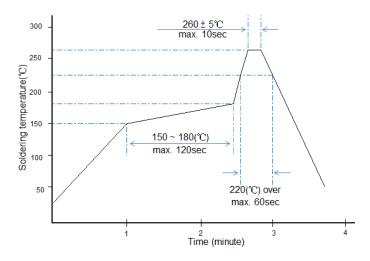
Recommended IR Reflow Soldering Profile
