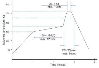
Recommended IR Reflow Soldering Profile MEET J-STD-020D
